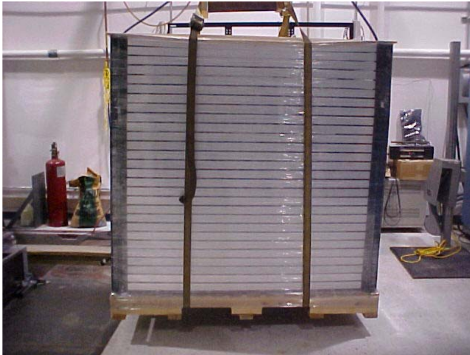
6-inch free fall drop setup
